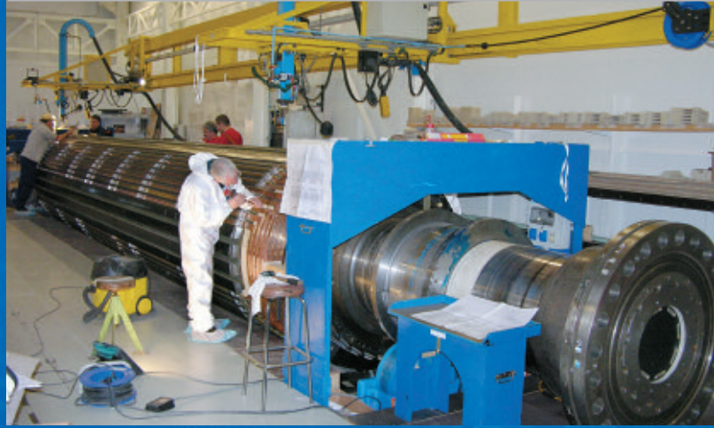
Overhaul of 80 MVA aircooled generator
