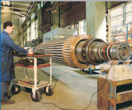
Test after rewinding 95 MVA rotor
