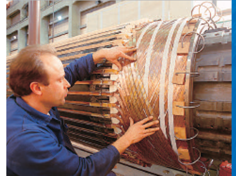
295 MVA JEUMONT generator (hydrogen-cooled)
