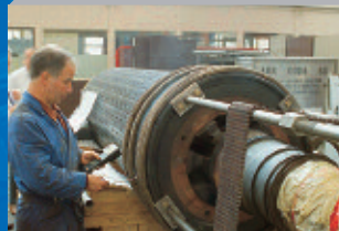
Reassembly of end bell on 80 MW rotor
